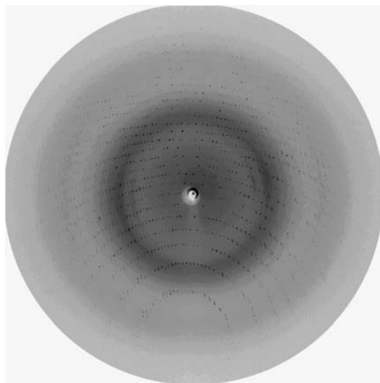
Figure 3 Diffraction image recorded for an EcAIII crystal. Crystal oscillation \Delta\varphi = 1.0^\circ . The maximum resolution at the edge of the detector is 1.65 Å.
